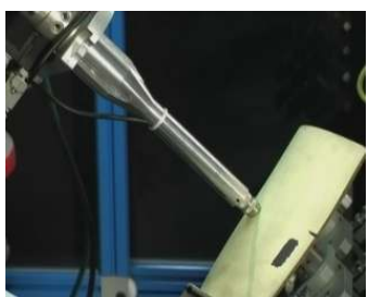
EDDY CURRENT INSPECTION
